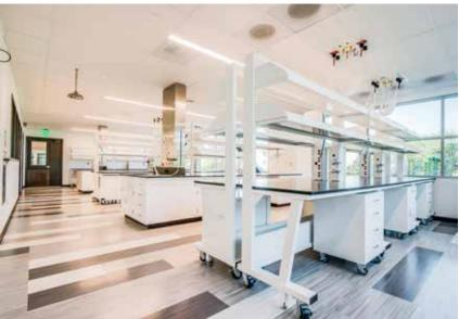
The lab space houses open chemistry lab space outfitted with numerous utilities, including emergency power, compressed air, local LN2 turrets, temperature monitoring ports for propriety and standard chemistry lab equipment. Tissue culture, clean rooms, fermentation rooms, clean and dirty Polymerase chain reaction rooms are surrounded by general labs and cold rooms.
